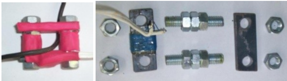
Figure 9: This inexpensive current transformer uses village-level technology, when connected to the microphone-input jack, it can measure AC amps (and by inference AC power)
