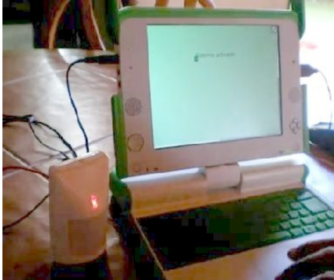
Figure 11: A pyroelectric sensor used for motion detection
